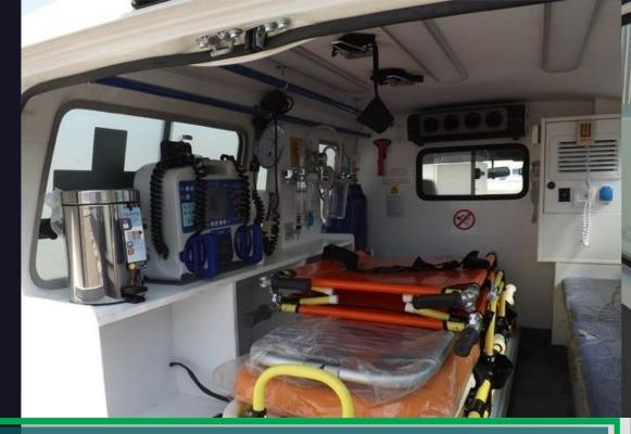
It is located on the left wall of the patient cabinet that oxygen tubes and oxygen suction system. The tubes are used as the average of 10\*2. Oxygen sockets are English type. The Ambulance oxygen system can be given as a French type oxygen system. It depends on the request of the customer. There is an external portable oxygen tube, which is one liter and a bag type. It works harmoniously with the ambulance ventilator system.
